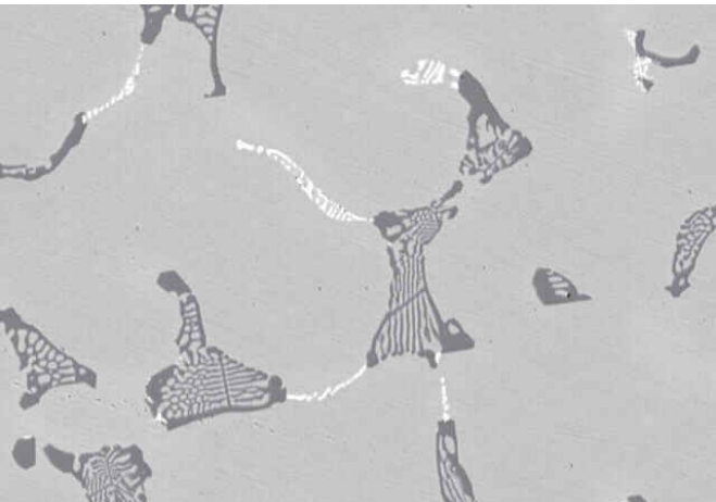
As cast structure of Manaurite® XTC. Black particles correspond to chromium carbides and white particles correspond to niobium or titanium carbides/nitrides.
